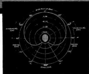
1. Cardioid directional response of 639A
